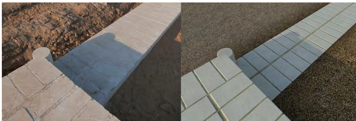
Figure 5. Calibration check using a photograph from on-site (left) and the simulated sunlight and shadows (right).
